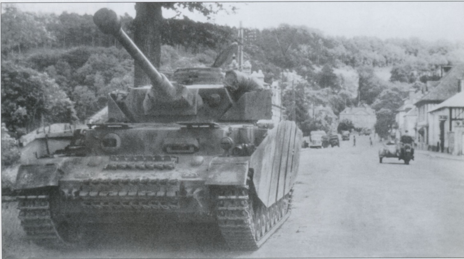
A new Pz.Bef.Wg.IV Ausf.H parked alongside a road leading through a French town on the way to the invasion front. A 2m 'Sternantenne D' (star antenna) for the Fu 8 radio set can be seen mounted where the normal antenna was mounted which, along with the lack of a tactical number on the turret skirt, would indicate this is probably a II.Bataillon command vehicle. Production of the Pz.Bef.Wg. IV started in March 1944 with 88 units being converted from rebuilt Panzer IV's. Records indicate that the division was issued with 5 on 30 April 1944. The divisional emblem of the 12.SS-Panzer-Division can be seen painted in white on the right mudguard.
